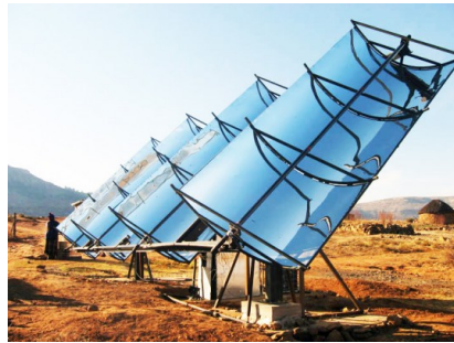
FIGURE 1 – Concentration solar panel Organic Rankine Cycle (Crédit STG international)
